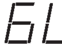
Active Protection – Code 6L – Compressor open start circuit
