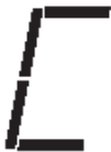
Flashing upper case C A call for second stage cooling has been received
