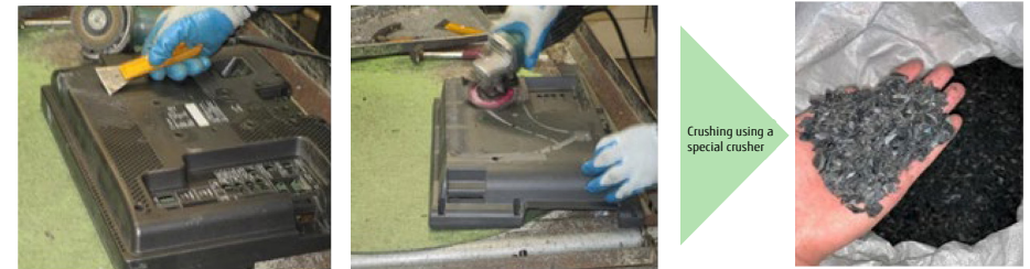
Removal of foreign substances (labels, metals, etc.) from cabinets
