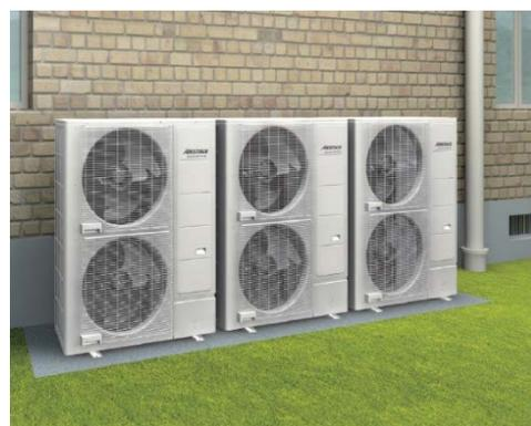
Furthermore, the new J-IIIIL models boast a large, 570mm propeller fan and a 15-120rps scroll compressor, ensuring low noise levels during operation. This enables units to be installed without the need for specialist soundproofing. Plus, Fujitsu's advanced refrigerant control technology allows for a maximum refrigerant piping length of 400m, opening up an array of system design and installation possibilities.
