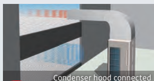
Condenser hood connected
