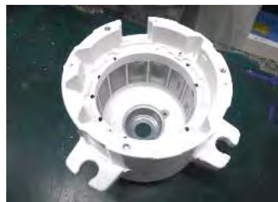
Wound coil component after BMC shaping
