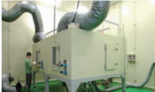
Calorimeter Measure the cooling/heating capacity by measuring the inlet and outlet temperatures, humidity, and air volume of the air conditioner.
