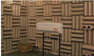
Silent Room Measure the operating sounds of air conditioners with the sound reflection-proof walls and ceiling.
