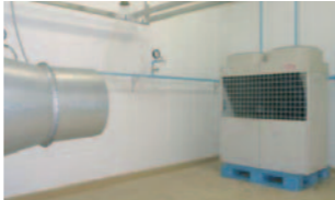
Shower Test Room Check on whether the electrical box of the outdoor unit is protected by rain waters with typhoon like wind.
