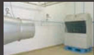
Shower Test Room Check on whether the electrical box of the outdoor unit is protected by rain waters with typhoon like wind.
