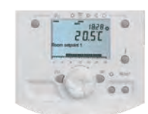
HMI Kit (option) UTW-KHMXE Supports multiple languages
