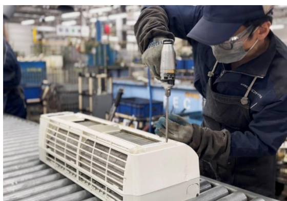
Manual disassembly of a used air conditioner
