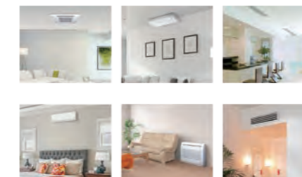
6 5-6 Rooms Multi Lineup of multi type for air conditioning from 2 rooms to 6 rooms with one outdoor unit in apartments where it is difficult to secure space for the installation of outdoor units
